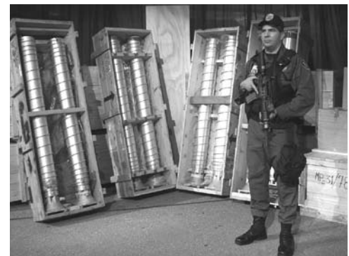
P-1 centrifuges recovered in Libya, similar in design to Iran's centrifuges at Natanz. Note the difference in scale from the gaseous diffusion units.
