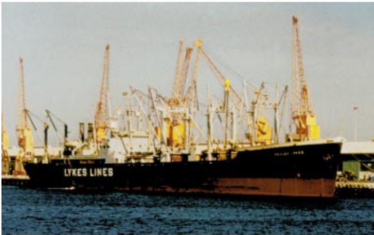
General cargo and breakbulk ships, while dated in terms of cargo loading and unloading operations, are militarily useful because of great flexibility and the capability to operate effectively through austere ports.
