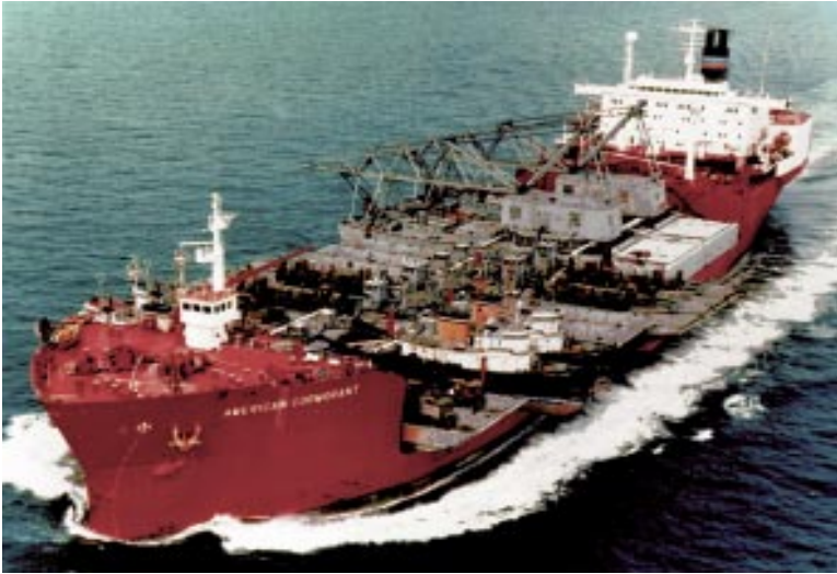
The heavy lift ship American Cormorant uses Float-on/Float-off capability to handle oversized military cargo.
